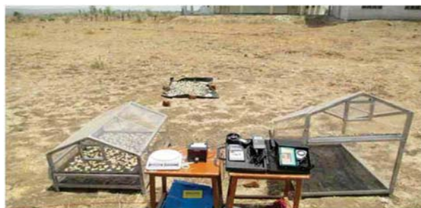
Fig. 2 Experimental setup in modified solar greenhouse dryer
