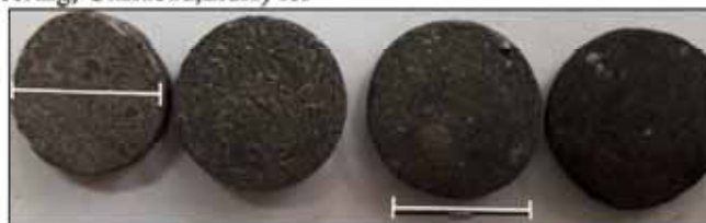
Fig. No. 3 Prepared titanium foam made by using +100 \mu\text{m} cenosphere mess size as spacerholder 50%,60%,70% and 80% volume fraction respectively
