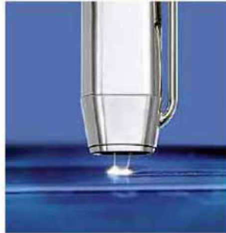
Fig No. 9: Tandem Wire GMAW with two wires in the same
