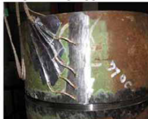
Fig No. 20: Thermocouple located on the inner surface of pipe
