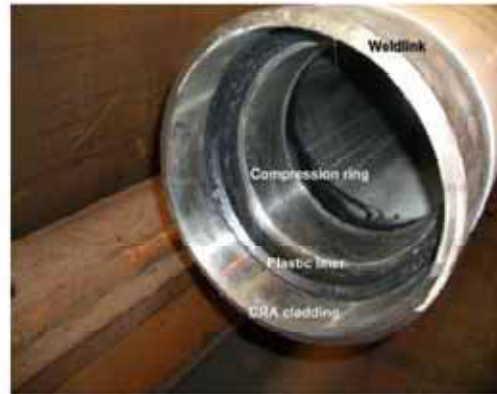
Fig No. 4: End of a stalk with weld link assembly
