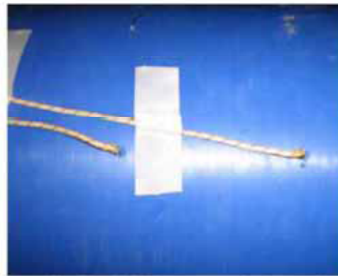
Fig No. 22: Thermocouples located on the outer surface of PBJ
