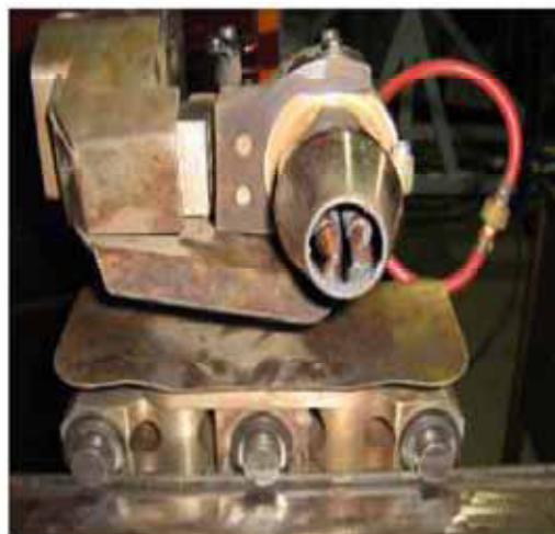
Fig No. 14: Tandem torch mounted on bug
