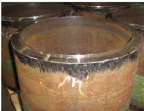
Fig No. 17: Ground and wire brushed pipe
