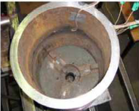
Fig No. 19: Thermocouples located on the outer surface of pipe
