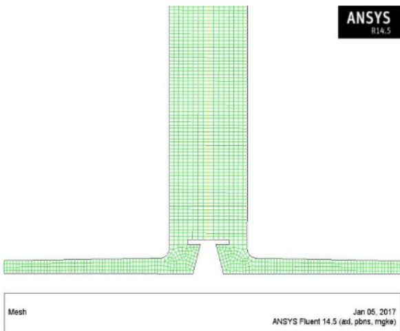
Fig.9 (b) Magnify view of Chimney height at 194.6 m
