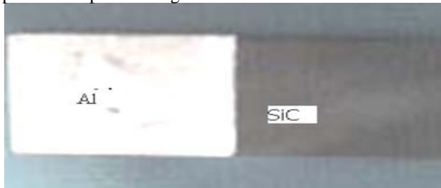
Fig 1: Al/SiC interface bonding.
