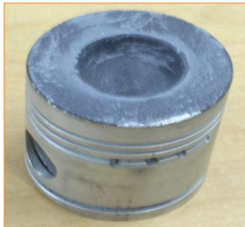
Fig 2 Piston with Sic coating using Plasma Spray process
