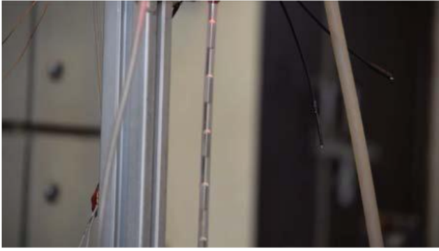
Fig. 2: picture showing slug flow regime in capillary at a liquid flow rate of 2LPH and gas flow rate of 0.5 LPH
