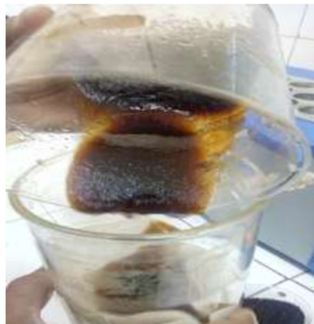
Fig. 1 - Recovered Glaubers Salt from mother liquor after filtration followed by air dyed/dried
