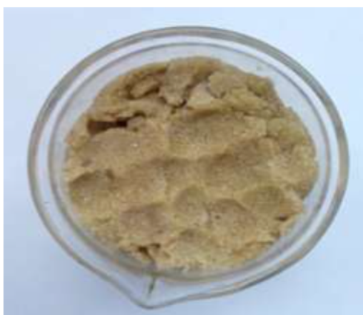
Fig. 4 - Recovered Glaubers Salt crystals from mother liquor
