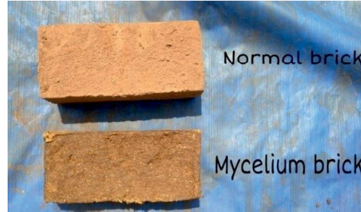
Fig.13 Normal brick and Mycelium brick
