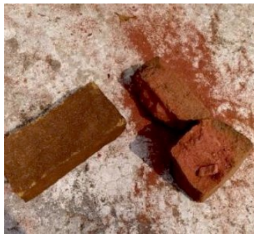
Fig. 14 Mycelium brick and normal brick dropped from 3 feet
