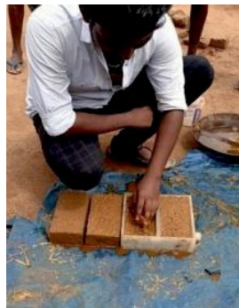
Fig. 11 Placing of grinded mixture in brick mould
