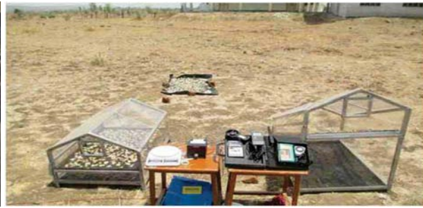
Fig. 2 Experimental setup in modified solar greenhouse dryer
