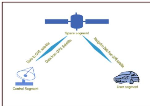
Fig. 3 Structure of GPS
