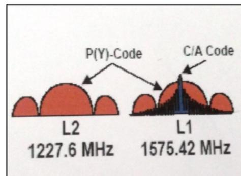
Fig. 5 Signal spectrum for current GPS signal
