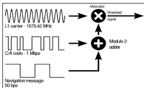
**Fig. 6 GPS signal spectrum**
